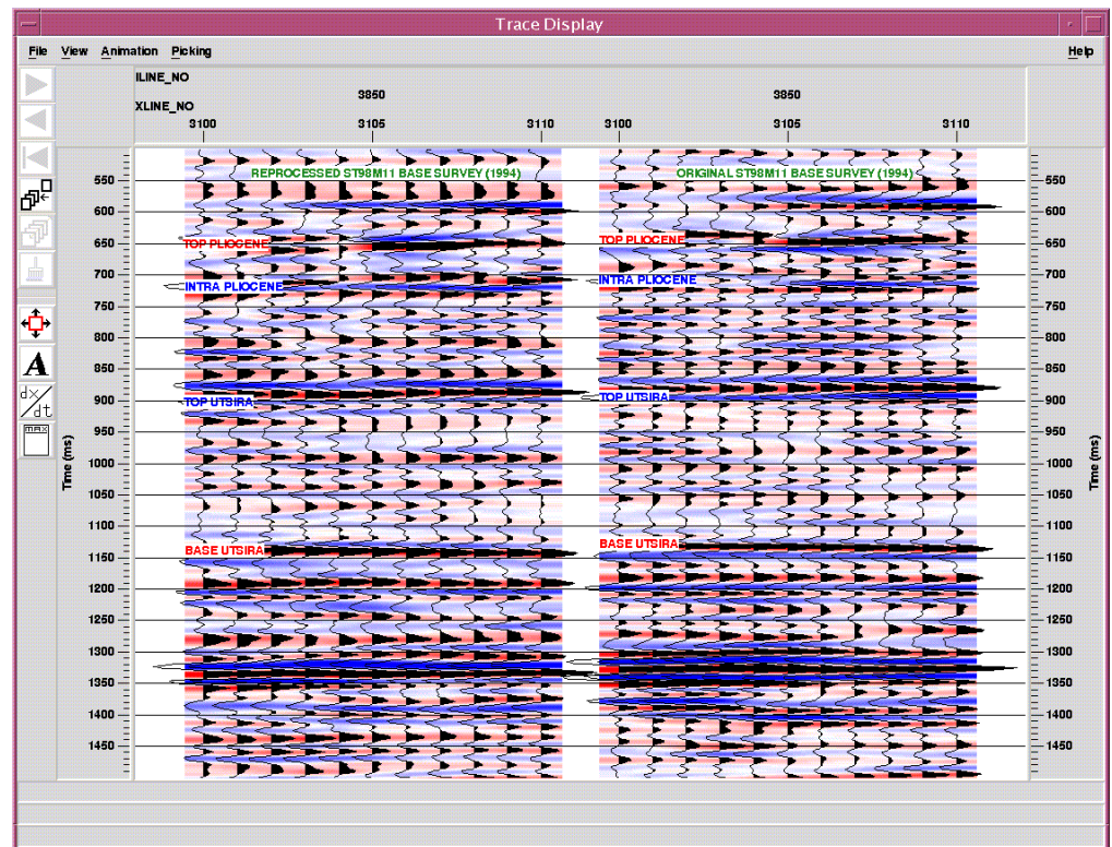
Figure 2: Time shift of approximately 8 ms between the 2 surveys with the reprocessed survey (left) “lower” than the original survey (right). Key horizons are indicated in the color of their polarity. The high energy reflections just above the Top Utsira sand are caused by tuning effects with the sand wedge reflections coming in from the east.
